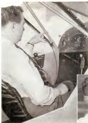
A two-finger lever control in the plane's cockpit sets the tail-wheel brake seen at right, for a quick stop
